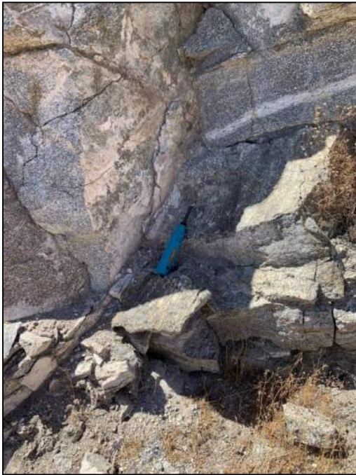
PHOTO 75: Closeup of granitic rock displaying east dipping foliated texture.
