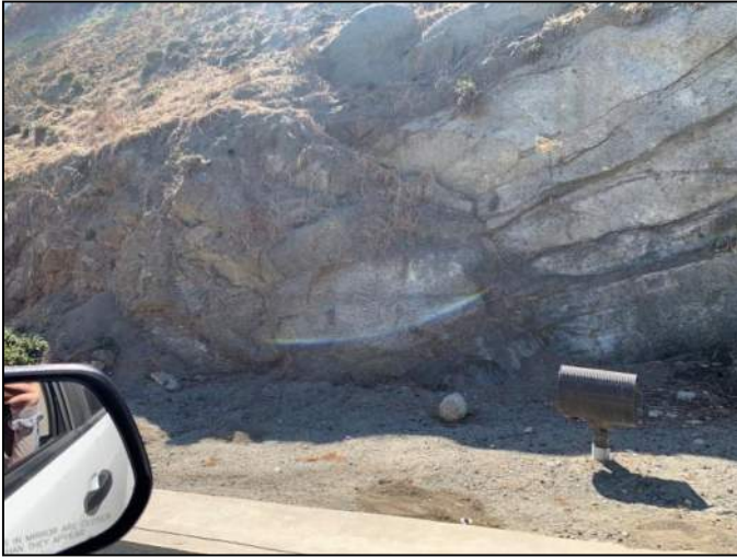
PHOTO 201: Outcrop of moderately weathered granitic rock near MP 78.8.
