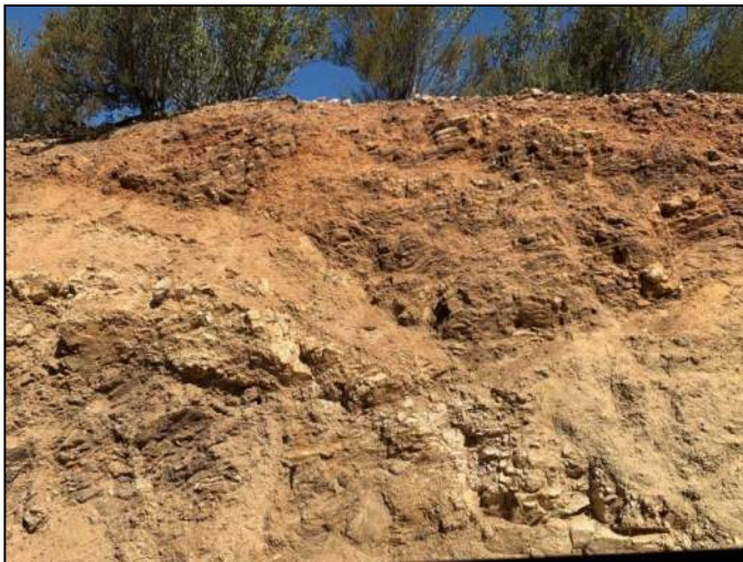
PHOTO 151: Highly weathered to decomposed metamorphic rock.
