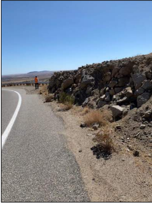
PHOTO 69: Moderately weathered granitic rock.
