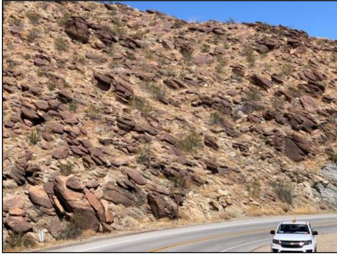
PHOTO 77: Outcrop of weathered granitic rock surface showing overall east dipping structure.
