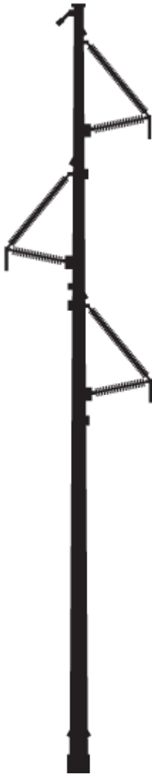
Fig: Typical steel pole tangent structure (230kV)
