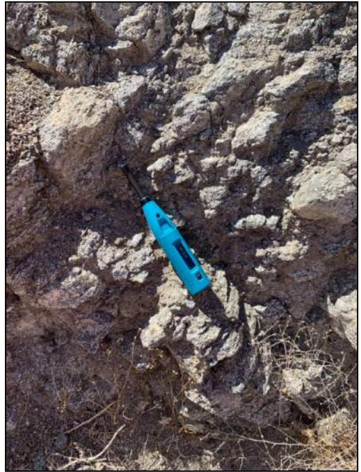
PHOTO 78: Outcrop highly weathered granitic rock.
