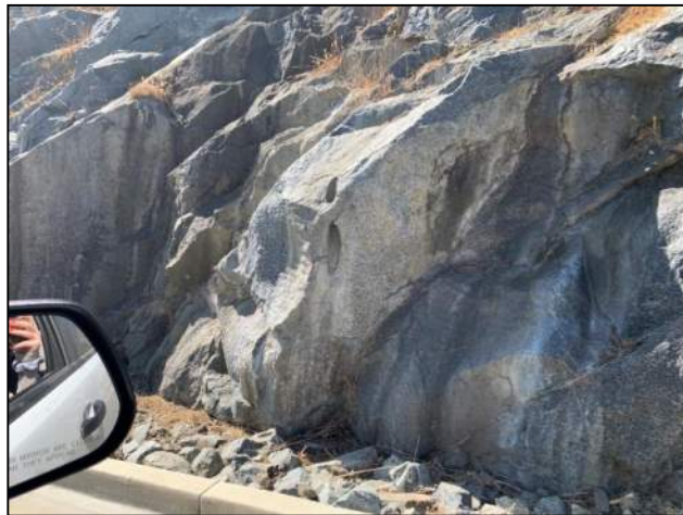
PHOTO 200: Outcrop of slightly weathered granitic rock on Nyemi Pass Place near Valley View Casino.
