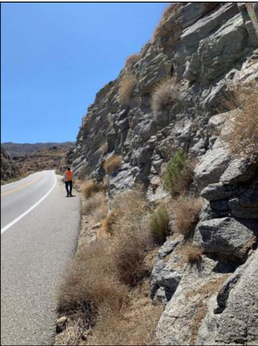
PHOTO 91: Moderately to slightly weathered granitic rock.
