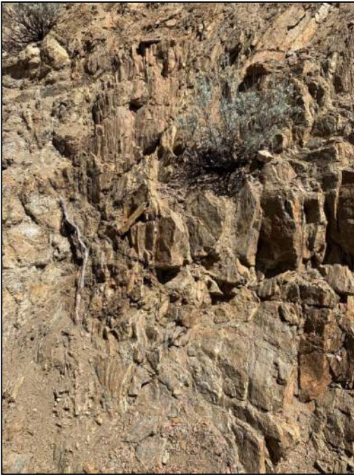
PHOTO 157: Highly weathered metasedimentary rock.
