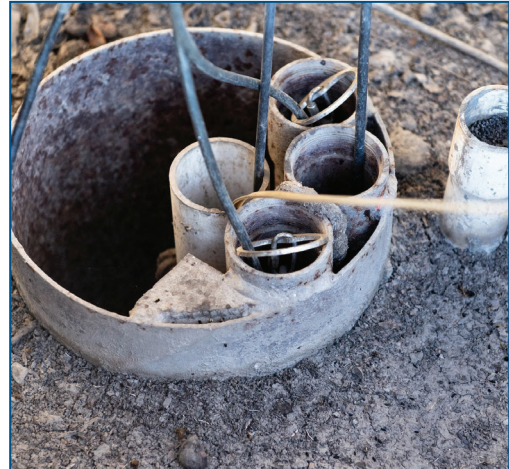
Monitoring wells are used throughout the state to measure groundwater levels.
